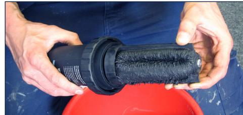
**UK CLEANING AND SERVICING** For optimum efficiency, clean out annually. Have a 750ml (min) container ready. Isolate heating system and close both valves. Open air vent (5). Using the spanner included in the pack open the drain valve. Drain all contents and then firmly close the
