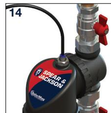
**UK CHEMICAL DOSING** Isolate boiler. Close isolation valves. Open drain valve to release air pressure (6). Close drain valve. Remove air vent screw (12) or fully remove air vent (13). Connect dosing device (14). Open outlet isolation valve. Apply dose (500ml max.). Close outlet isolation
